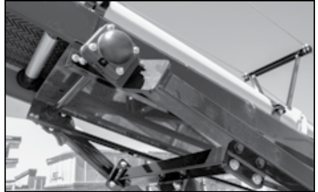
Fig 56 - Upper lift bearings
