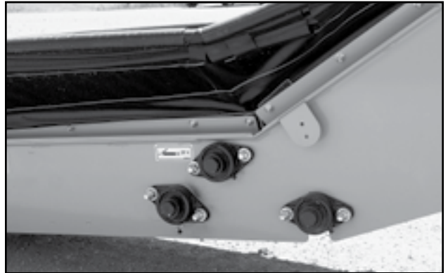
Fig 50 - Transition roller bearings
