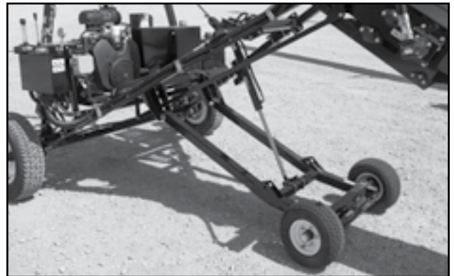
Fig 14 - Steering wheels with cylinder
