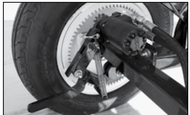
Fig 24 - Disengage drive wheels
