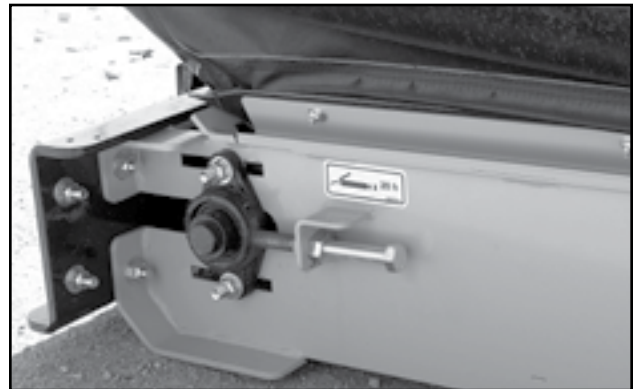
Fig 45 - Tail roller bearing
