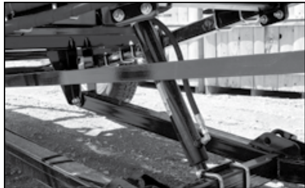
Fig 54 - Steering wheel lift cylinder
