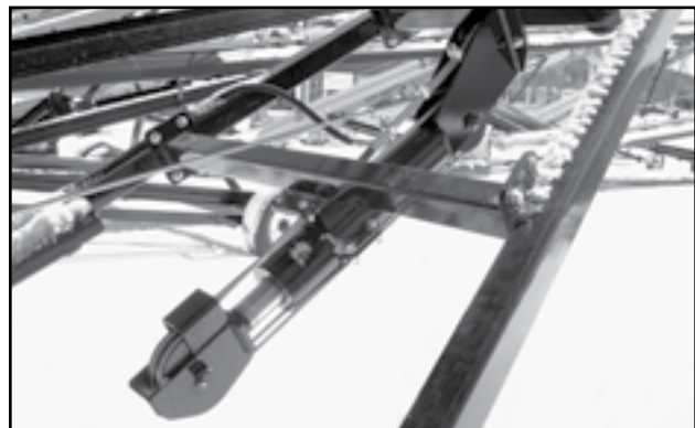
Fig 55 - Conveyor tube lift cylinder
