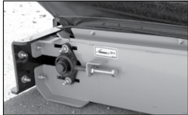
Fig 60 - Tail roller with adjustment bolt
