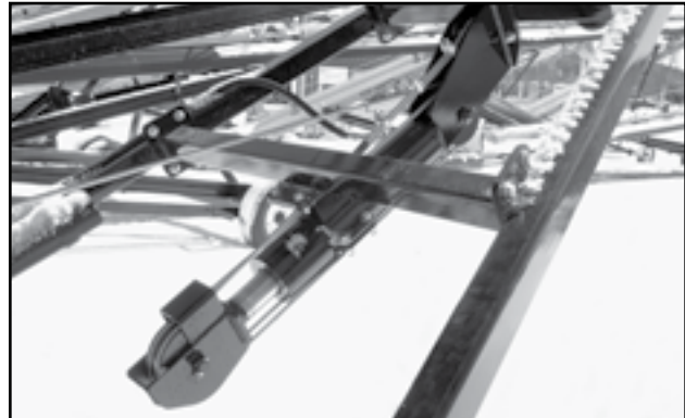
Fig 16 - Tube lift cylinder
