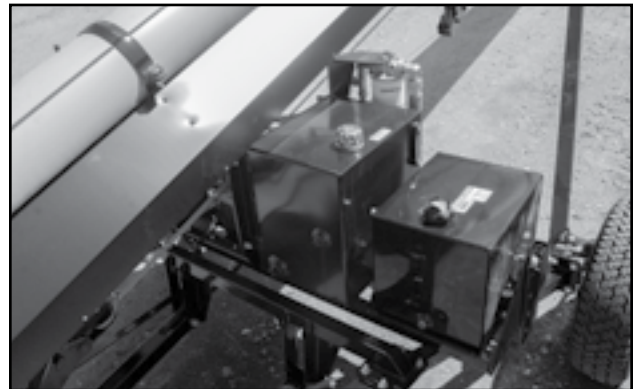
Fig 8 - Fuel tank and hydraulic reservoir
