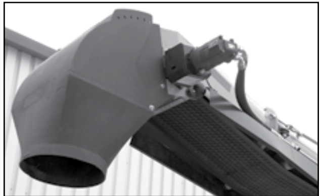
Fig 51 - Drive and discharge roller bearings
