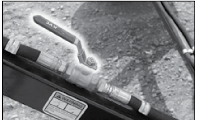
Fig 30 - Hydraulic ball valve to lift cylinder
