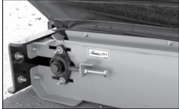
Fig 46 - Adjustment bolt on tail roller
