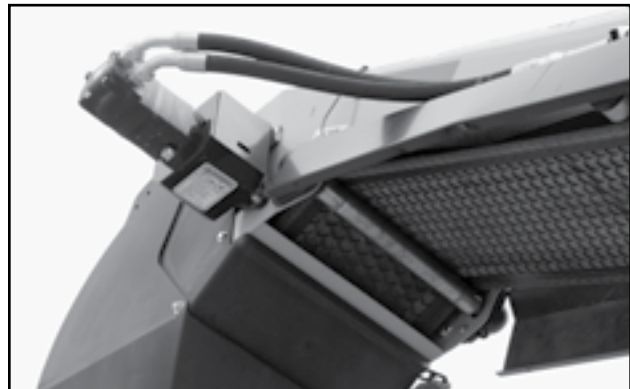
Fig 48 - Hydraulic motor, conveyor belt drive
