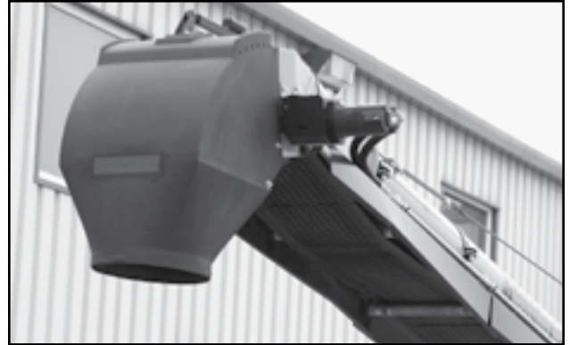
Fig 12 - Discharge spout and hydraulic motor
