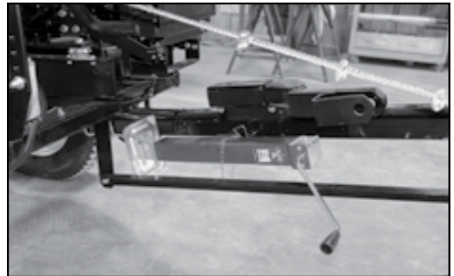
Fig 36 - Hitch and jack storage plate
