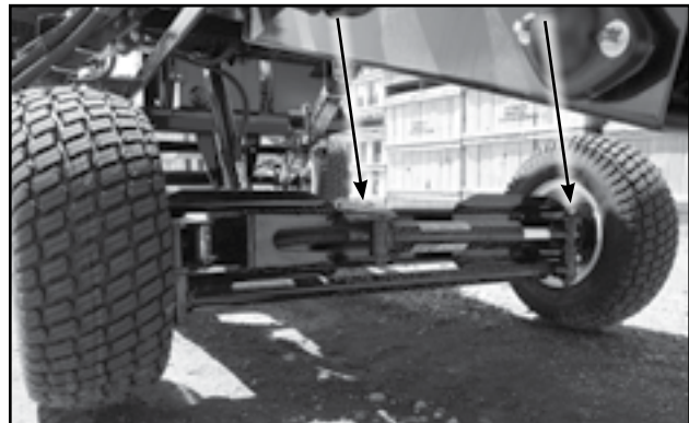
Fig 53 - Steering wheel axle bushings
