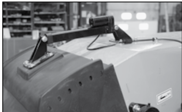
Fig 18 - Electric actuator on discharge spout
