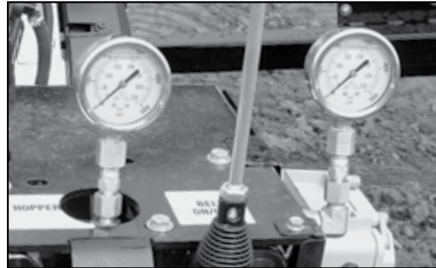
Fig 10 - Hydraulic pressure gauges
